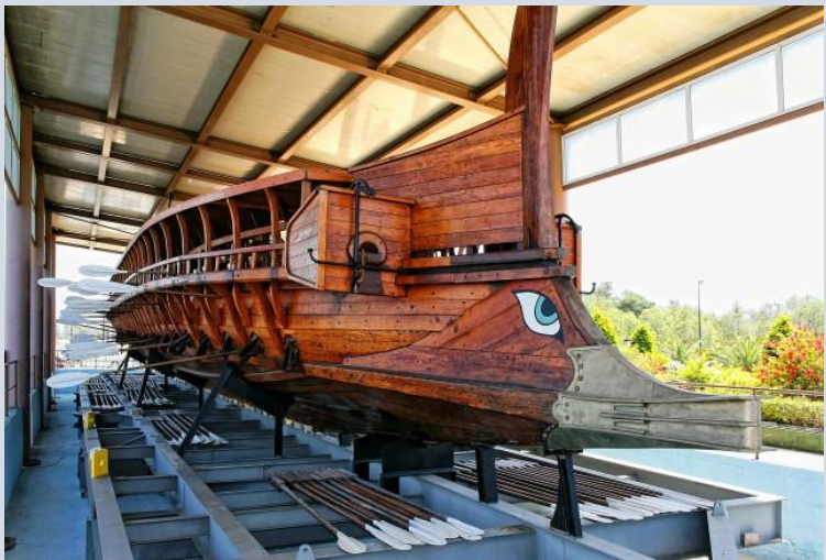
A modern reconstruction showing the bronze ram as well as a basic eye design used for intimidation
