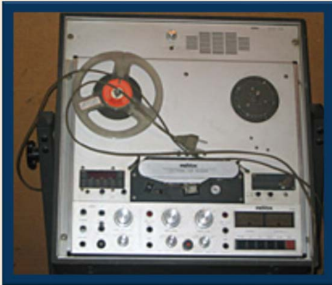
ReVox quarter-inch reel-to-reel recording equipment.
