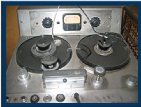
Ampex quarter-inch reel-to-reel recording equipment.
